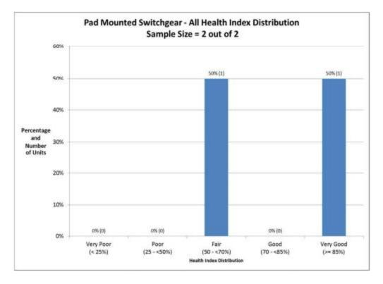
Figure 5.3-12: Pad Mounted Switchgear HI Results
