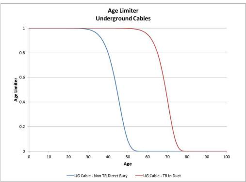
Figure 5-1 Age Limiting Factor Criteria - - Underground Cables
