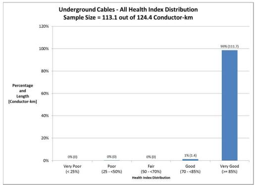
Figure 5-3 Health Index Distribution - Underground Cables
