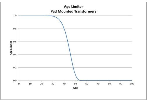
Figure 2-1 Age Limiting Factor Criteria - - Pad Mounted Transformers
