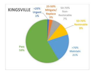
Overall, the trend shows 9% of the poles inspected will require mitigation or replacement. If the trend continues, just under half of those poles that require replacement will require *urgent* replacement. This high percentage will reduce in future inspections, as the bulk of the defective poles will already be replaced. The number of poles to be inspected that are pre 2000 is unknown. It is estimated that it will be 55 – 80% of the poles in service.
