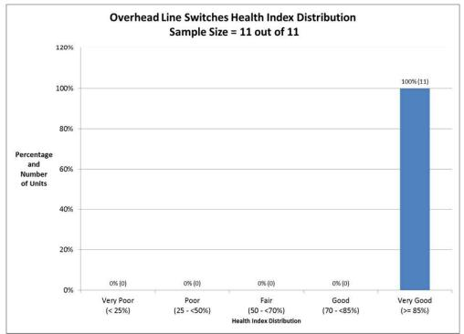
Figure 3-3 Health Index Distribution - Overhead Line Switches
