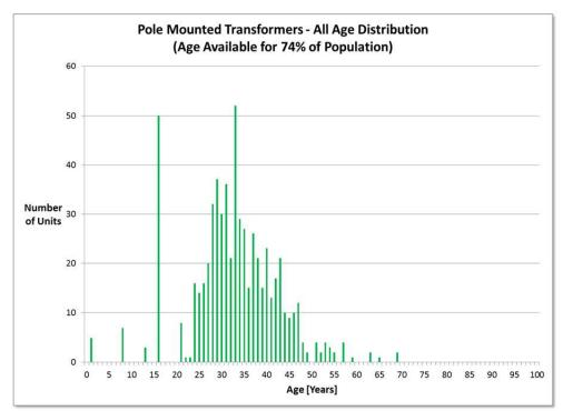
Figure 1-2 Age Distribution - Pole Mounted Transformers
