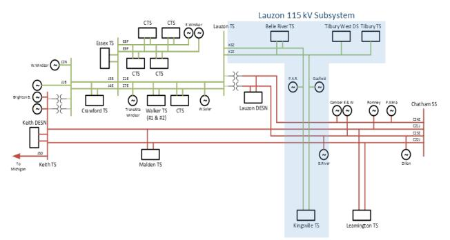
Figure 6-3: Lauzon 115 kV Subsystem
