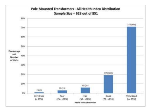
Figure 5.3-6: Pole Mounted Transformer HI Results
