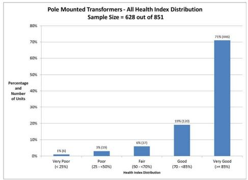
Figure 1-3 Health Index Distribution - Pole Mounted Transformers
