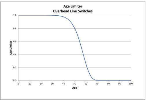
Figure 3-1 Age Limiting Factor Criteria - - Overhead Line Switches
