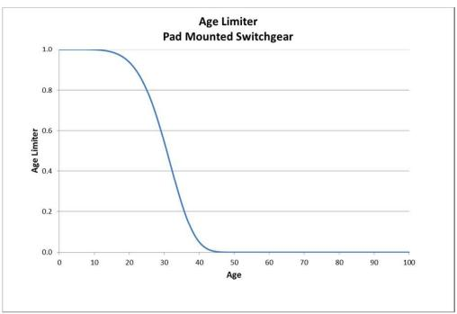
Figure 4-1 Age Limiting Factor Criteria - - Pad Mounted Switchgear
