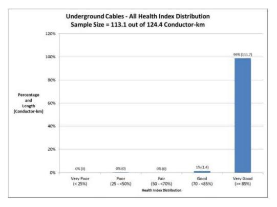
Figure 5.3-14: Underground Cable HI Results
