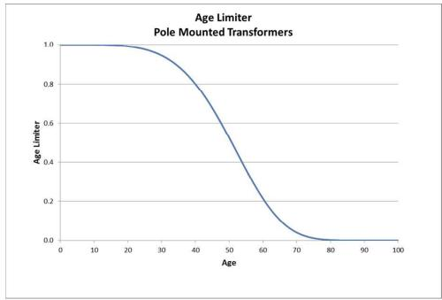
Figure 1-1 Age Limiting Factor Criteria - - Pole Mounted Transformers
