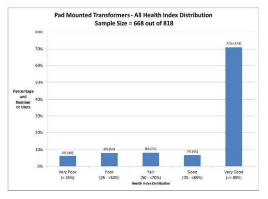
Figure 5.3-8: Pad Mount Transformer HI Results
