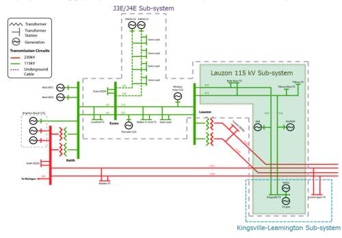
Figure A-2: Single Line Diagram of Electricity System Supplying the Windsor-Essex Region
