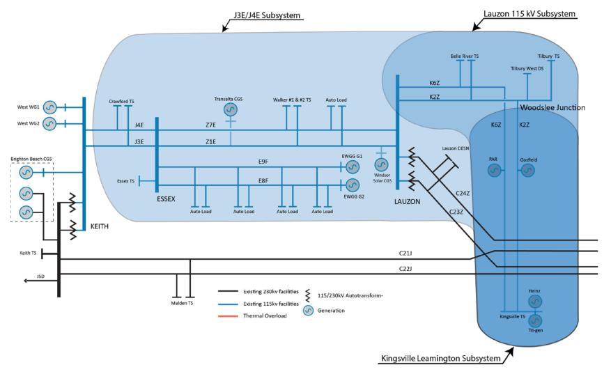
Figure 2. Windsor-Essex Region Subsystems/Single Line Diagram
