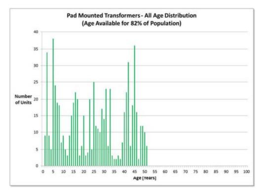
Figure 5.3-7: Pad Mounted Transformer Age Demographic
