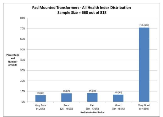
Figure 2-3 Health Index Distribution - Pad Mounted Transformers
