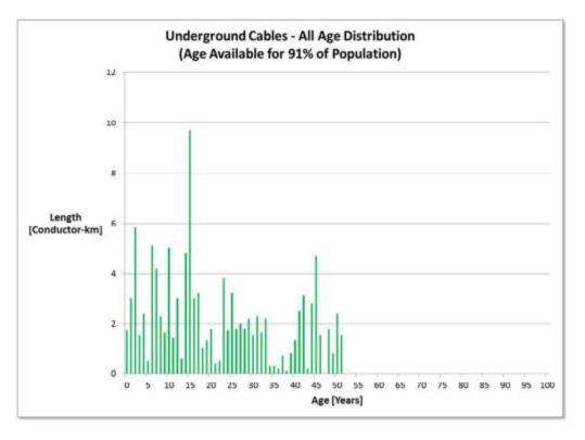
Figure 5.3-13: Underground Cable Age Demographic
